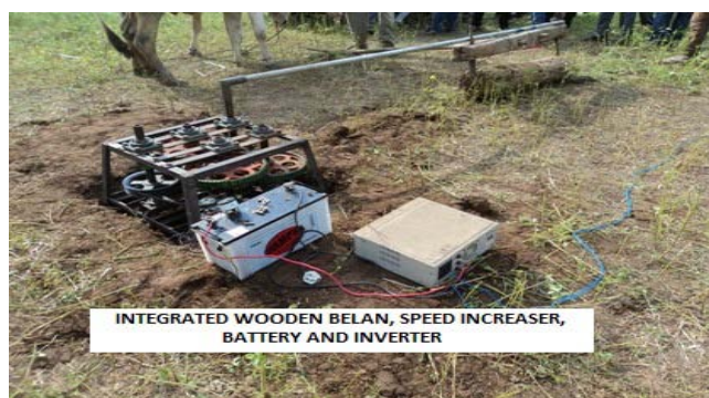
Fig. 3: Integreted Belan, Speed Icreaser, belt&pulley, alternator and battery.
