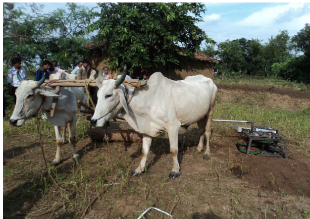
Fig. 4: Mechanical device for generating power using animal power.
