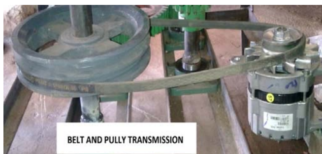
Fig. 2: Belt and pulley unit of speed increaser.
